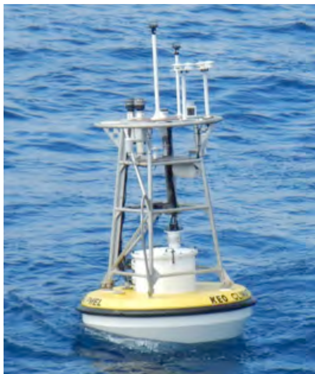
Figure 2. Typical OCS surface mooring configuration.
