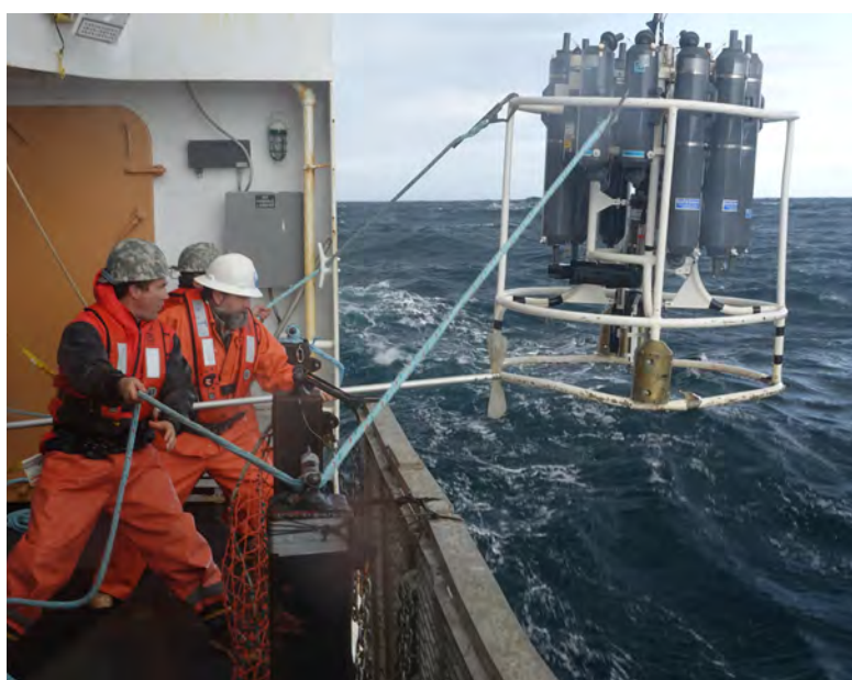
Figure 2. Crew of the NOAA Oscar Dyson retrieve a CTD in the Eastern Bering Sea during an EcoFOCI research cruise in 2016. A CTD is an oceanographic instrument that captures the conductivity, temperature and depth as it is lowered and raised at set locations into the water alongside the vessel. The bottles capture water samples at various depths that are used for further analysis.
