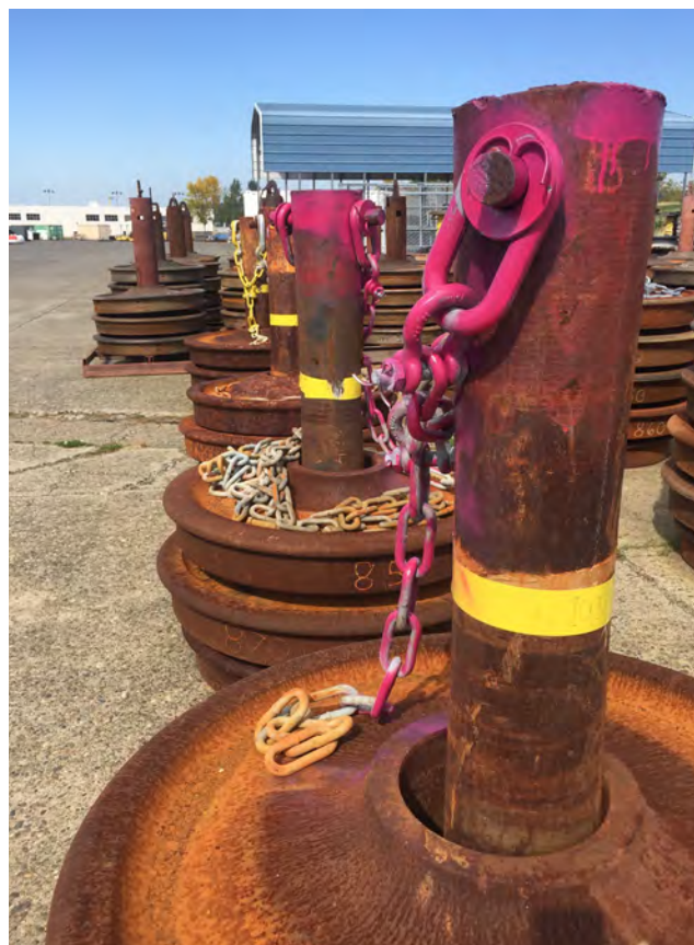
Figure 3. How do moorings stay in the same place? Railroad wheels! EcoFOCI maintains a biophysical mooring array in the Bering and Chukchi seas, and each year during deployment, these anchors are used to keep the moorings in place. These are the railroad wheels just after delivery at the NOAA western regional campus.
