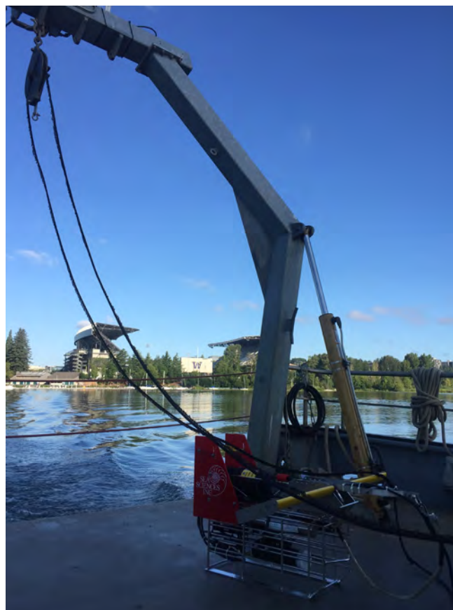
Figure 1. EcoFOCI scientists use the UW APL Robertson to field test a towed platform, Acrobat, a lightweight and versatile towed body oceanographic research platform for high-resolution surveys of biological, physical and chemical processes in ecosystems. This equipment was used in the Bering and Chukchi seas in 2016.
