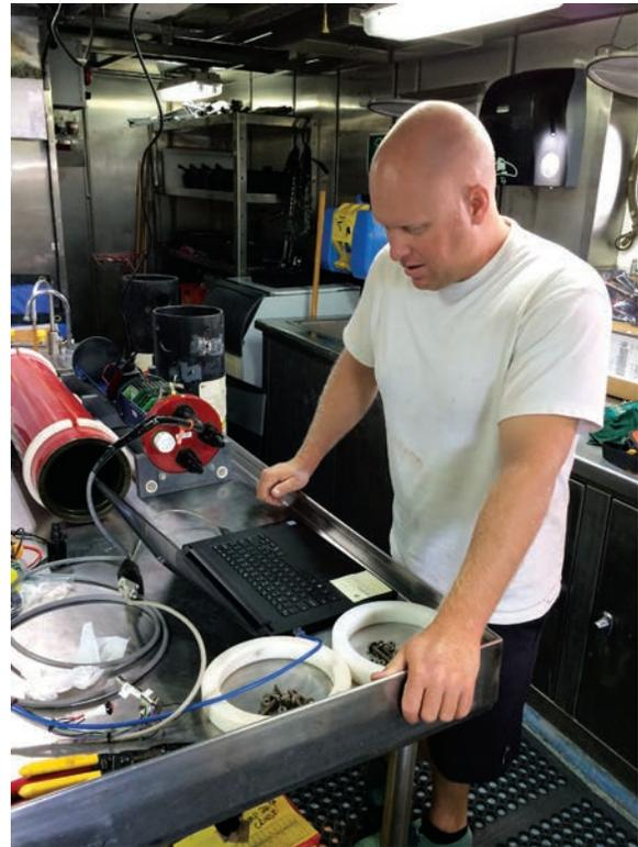
Figure 1. Erik Norris prepares a High-frequency Acoustic Recording Package (HARP) for deployment.
