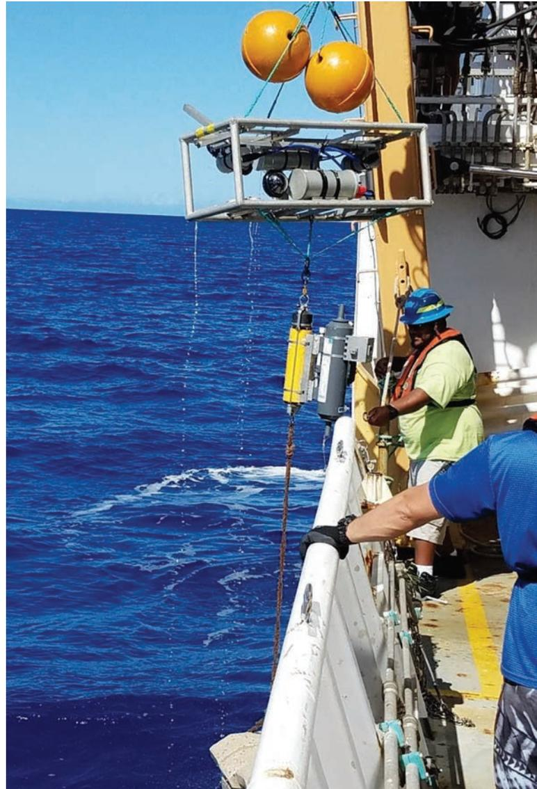
Figure 5. JIMAR customized eDNA sample bottle (with sample) being recovered by crewmembers of NOAA Ship *Oscar Elton Sette* as part of a DropCam Instrument Package (DCIP) deployed during the Bottomfish Fishery-Independent Survey-Hawaii (BFISH) 2018.
