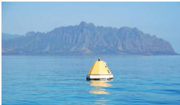
*Figure 1. The CRIMP-2 MAPCO<sub>2</sub> buoy has been making automated measurements of inorganic carbon system parameters on the barrier reef of Kaneohe Bay, Oahu, Hawaii since June 2008. Kualoa Point, a spur of the Koolau Range can be seen in the background.*
