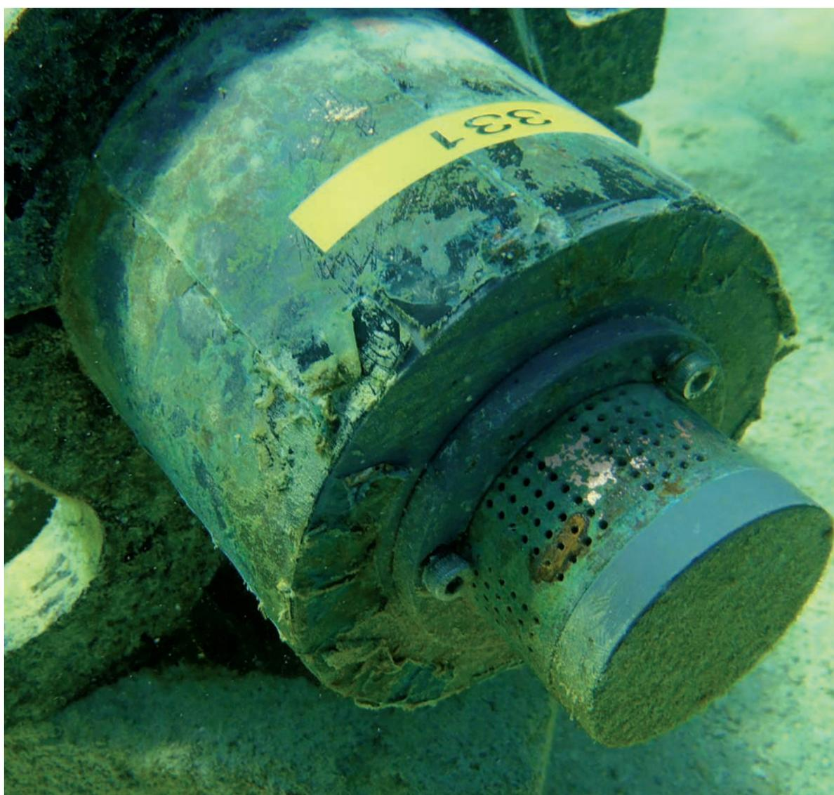
Figure 2. Close up of a SeaFET pH sensor showing evidence of biofouling.
