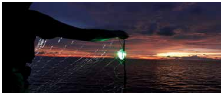
Figure 1. Green light LED being tested in Indonesian gillnet fisheries to reduce sea turtle bycatch.
